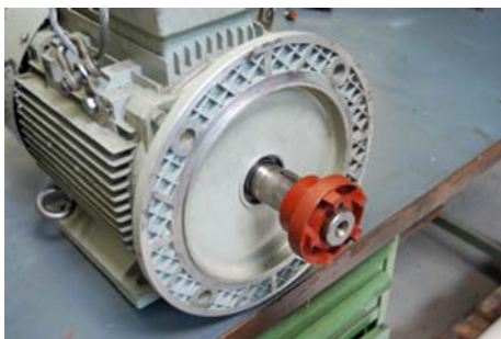
Fig. 27: Coupling half pushed onto the motor shaft
