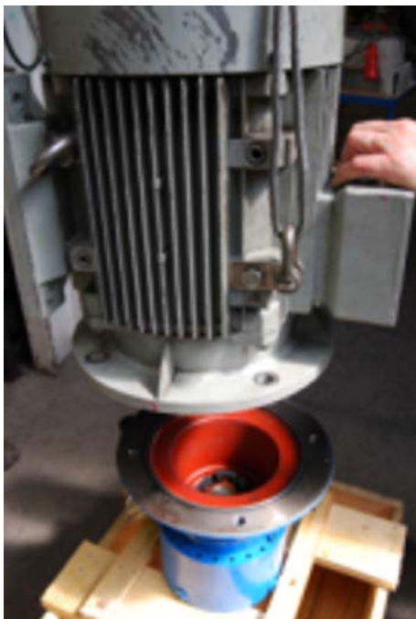
Fig. 32: Mounting the motor
