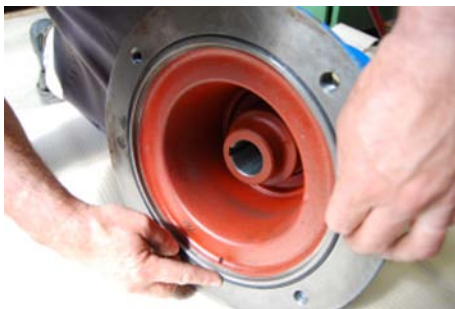
Fig. 31: O-ring inserted in the intended groove
