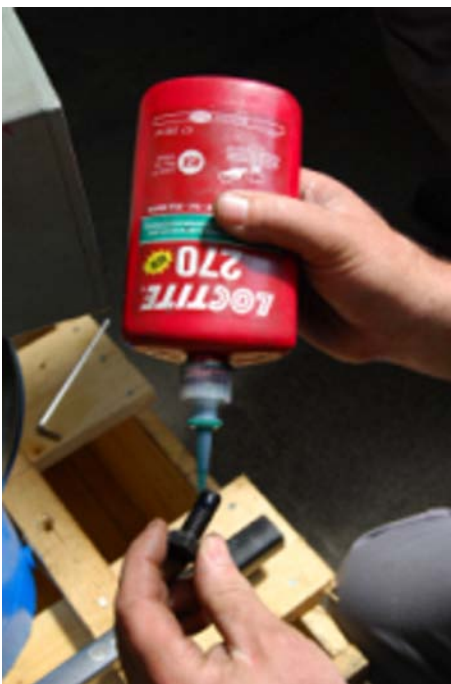
Fig. 35: Apply thread-lock compound to the bolts
