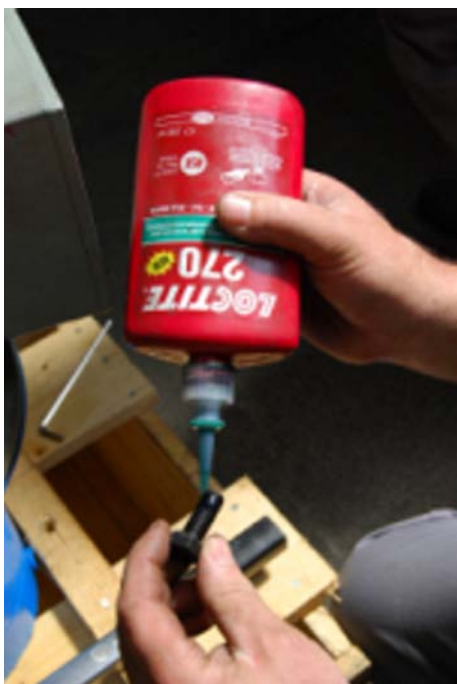
Fig. 33: Apply thread-lock compound to the bolts
