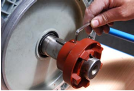
Fig. 30: Coupling half axially fixed in place
